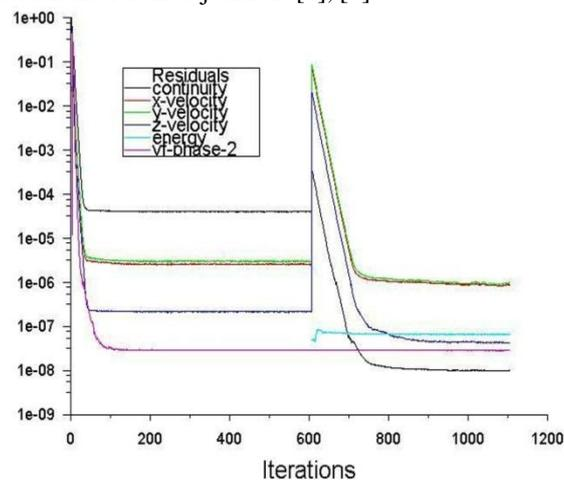
*Figure 2. Residuals of various flow parameters*
