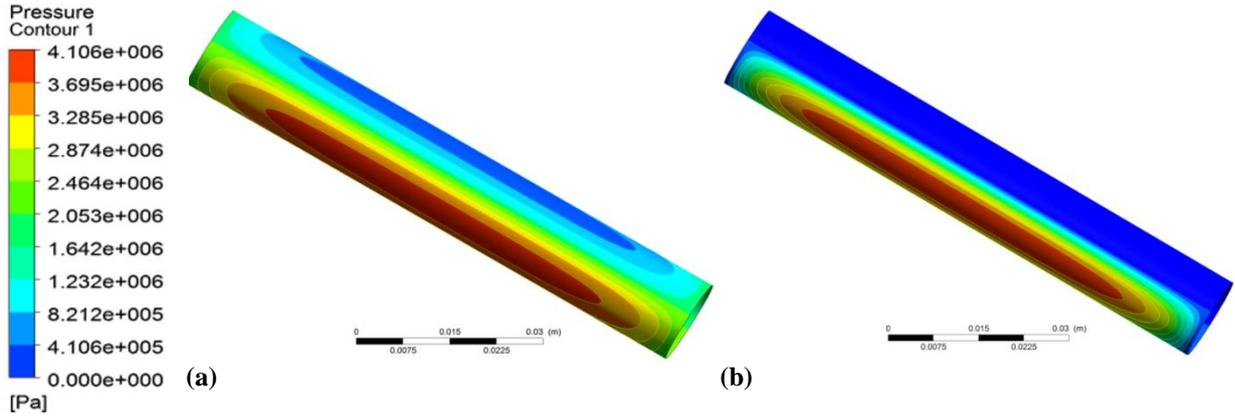
Figure 3. Pressure contours on the journal surface (a) without cavitation (b) with cavitation
