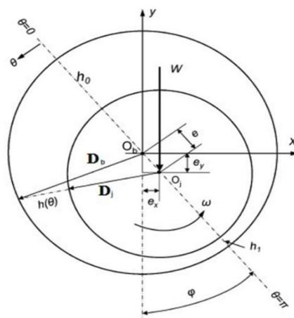
Figure 1. Schematic representation of the journal bearing
