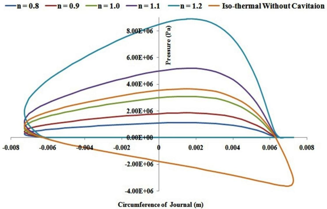
Figure 4. Pressure distribution at mid plane across the circumference of the journal for various flow index
