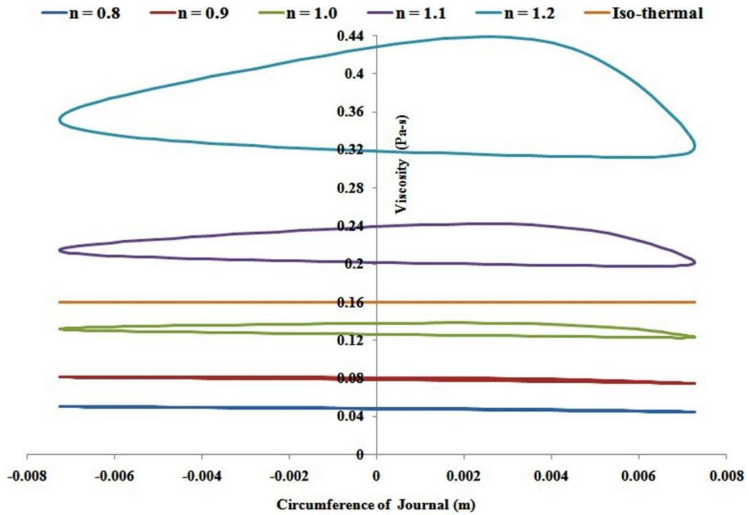
Figure 5. Viscosity distribution at mid plane across the circumference of the journal for various flow index
